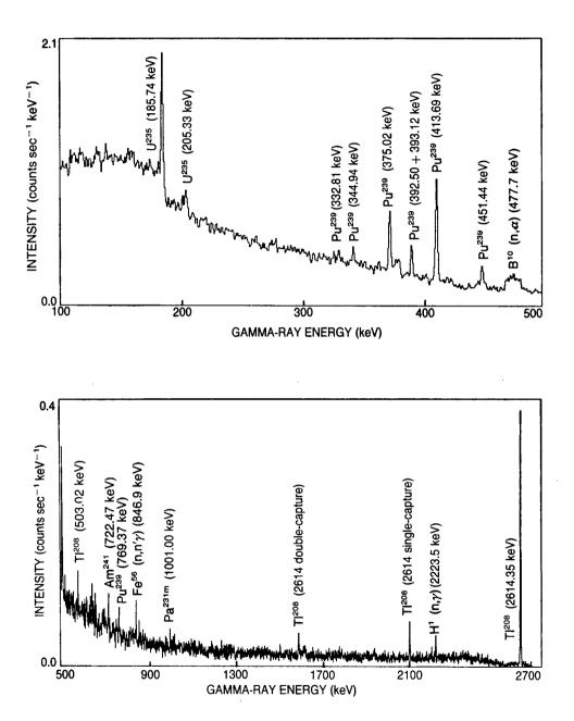
Figure 1: The gamma-ray signal recorded by a germanium detector placed on top of a cruise-missile launcher 3.4 meters from the lid for 10 minutes
