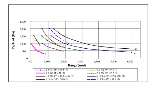
FIGURE 4-12 Payload versus ballistic range capability for notional two- and three-stage Submarine-Launched Global Strike Missile (SLGSM) configurations. All vehicles are constrained to a length-to-diameter ratio of 12. The number in parentheses indicates the number of missiles that can fit in a single launch tube of a nuclear-powered guided missile submarine.
