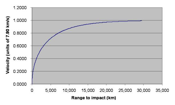
FIGURE G-2 Normalized velocity versus. range (Columns C versus E of Table G-1) for pure glide.
