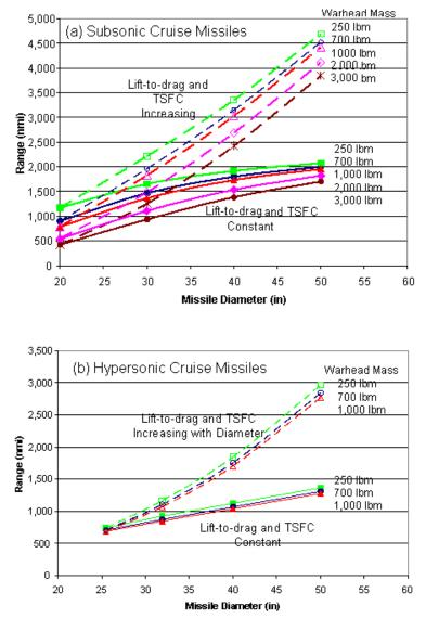
FIGURE 4-14 The impact of missile diameter and payload on range of notional (a) subsonic and (b) hypersonic cruise missiles. The solid curves are based on flight- or laboratory-demonstrated aerodynamic and propulsion technology. The dashed curves illustrate the potential performance improvements that result from potential aerodynamic and propulsion efficiency gains. NOTE: TFSC, thrust specific fuel consumption.
